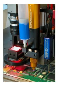
applications where the close proximity of the nozzle to the component risks direct contact and potential component damage between the part and the dispensing system, jetting serves as a viable alternative to traditional nozzle dispensers.
