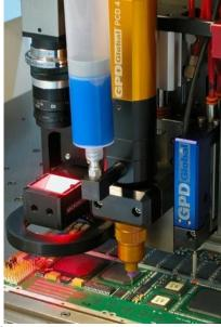
in mobile devices, wearable electronics, and advanced packaging. Additionally, in applications where the close proximity of the nozzle to the component risks direct contact and potential component damage between the part and the dispensing system, jetting serves as a viable alternative to traditional nozzle dispensers.
