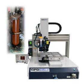
Time Pressure Liquid Dispensing Pump on Benchtop Dispenser and automated platform environments.
