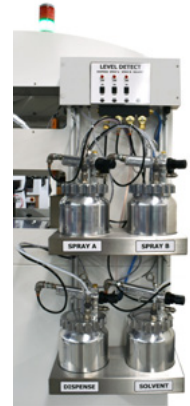
Multiple Reservoirs with Level Detect (option)
