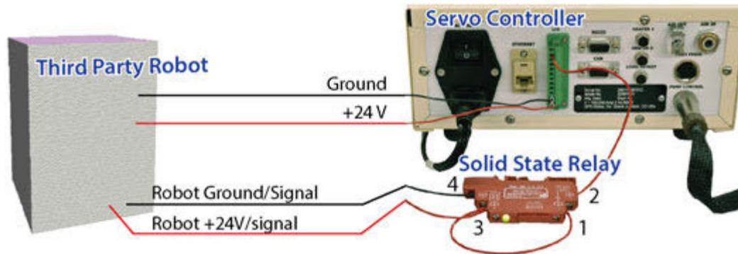
1. Route ground from controller I/O 11 to robot ground.
