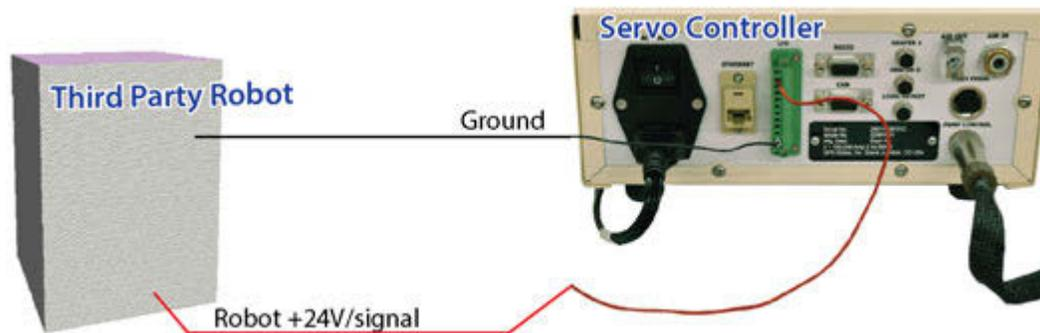
1. Route ground from controller I/O 11 to robot ground.
