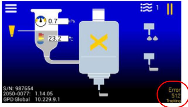
**TIP:** Motor control type errors may be displayed in multiples. For example: Tracking, Phasing
