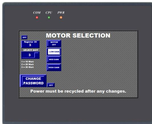
The parameters are only visible if the selector switch, in the top left column, is moved to the ON position.
