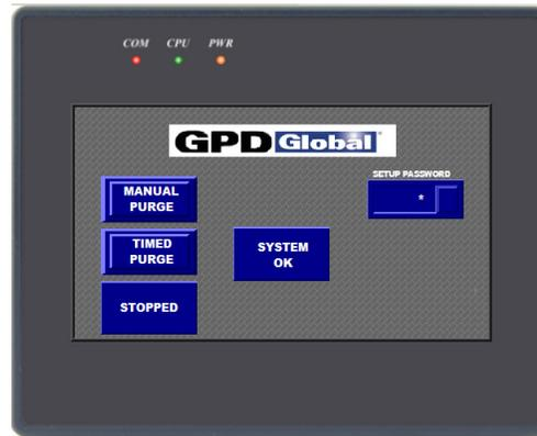
Initially, the GPD Global logo displays. The Main Screen displays 15 to 20 seconds after the power switched is turned on.
