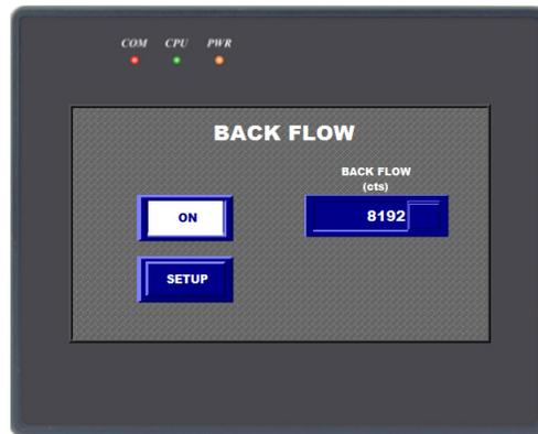
The Back Flow screen enables the user to force the pump to reverse the flow for a defined number of counts, after the pump move has been completed. The Back Flow draws back excess material away from the dispensing tip.
