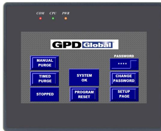
3. Now press the SETUP button. The SETUP screen will display.
