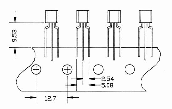
905-1CA TO BE USED WITH 0.76-1.14 P.C. BOARD HOLE DIAMETERS
