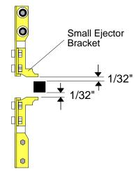
Figure 12 Adjust Small Ejector Bracket
