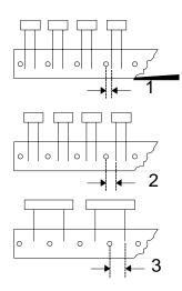
**Figure 15** Component Position Relative to Tape Hole
