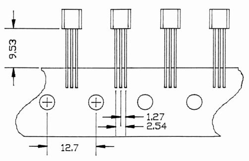
\* DIE 905-1E3 IS AVAILABLE FOR FORMING ALL LEADS IN LINE AT 90° WITH A MIN. (A) DIMENSION OF 2.03.
