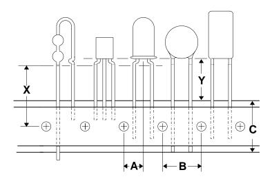
Figure 22 GPD's CF-9 Taping Specifications
