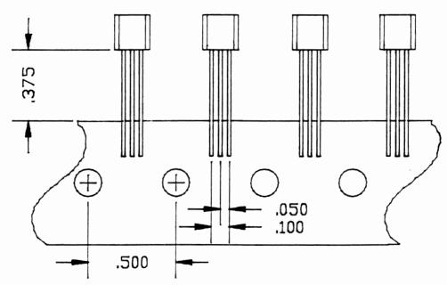
\* DIE 905-1E3 IS AVAILABLE FOR FORMING ALL LEADS IN LINE AT 90° WITH A MIN. (A) DIMENSION OF .080.
