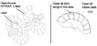
11. Apply glue. Sparingly apply Loctite's Black Max 380 or 454 Surface Adhesive to each transport wheel segment. Use light pressure to avoid warpage.
