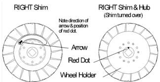
c. Install the flat wheel holder on the each shim loosely - DO NOT tighten the screws at this time.
