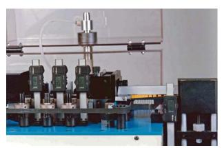
**Micrometer adjustment** included with every CF-10. Allows the operator to quickly set up the CF-10 to the correct setting for forming or cutting radial component leads.
