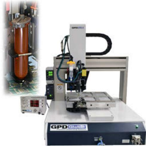
Monitor your Time Pressure Dispensing Pump with either a simple & versatile controller or an advanced FPC controller.
