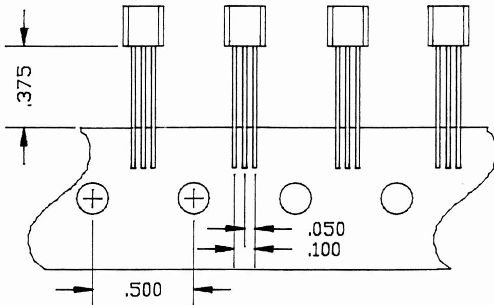
\* DIE 905-1E3 IS AVAILABLE FOR FORMING ALL LEADS IN LINE AT 90° WITH A MIN. (A) DIMENSION OF .080.
