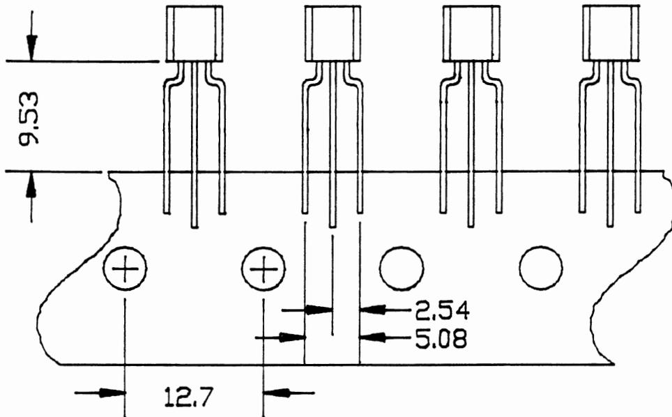
905-1CA TO BE USED WITH 0.76-1.14 P.C. BOARD HOLE DIAMETERS
