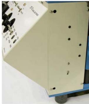
2 - Lay panel down to reveal sensor.
