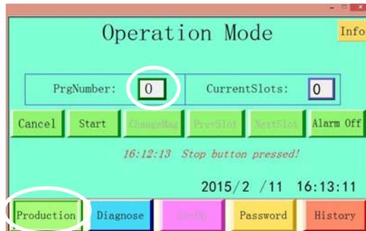
3. When the production interface opens, select the START button to start automatic production mode. The machine will home, get a magazine, move the magazine to the programmed position, and then proceed with automatic operations. The green light signal turns on
