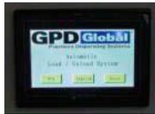
There is a color touch screen at the top of the machine. The operator can access it on the front of the machine. It is used to operate the machine and display machine status and information.
