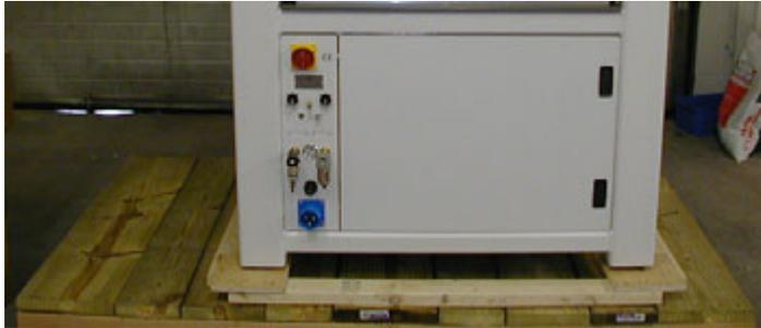
5. Adjust the machine feet downward as far as possible while still allowing space for wooden wedges (installed during the next step). Tighten all jam nuts on each foot before installing the wedges.
