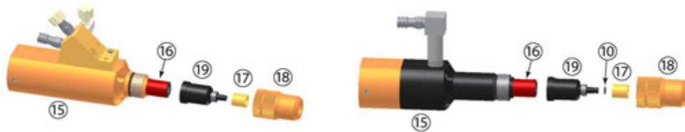
2. To unscrew the stator (Item 16) from the dispenser housing (Item 15) without separating the pin (Item E) mounted on the stator:
