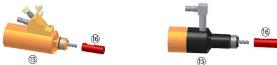
4. Carefully and thoroughly clean the stator (Item 16) using swabs supplied in the cleaning kit. Remove all debris; anything less than a thorough cleaning can affect pump performance.
