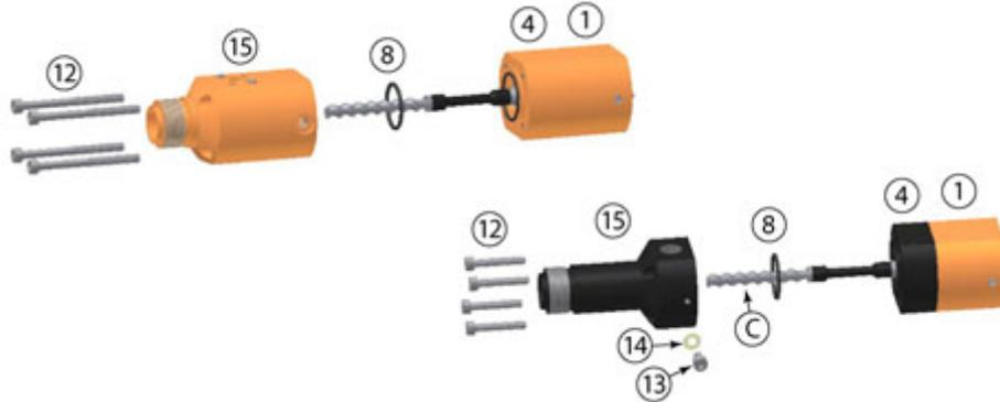
2. Remove screws (Item 12) and then separate dispenser housing (Item 15) from “bearing housing with rotor” assembly (Items 1 and 4).
