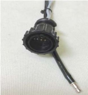
**Figure 2-3: 28-pin Jet Cable and Quick-Disconnect Jet Pressure Connector**
