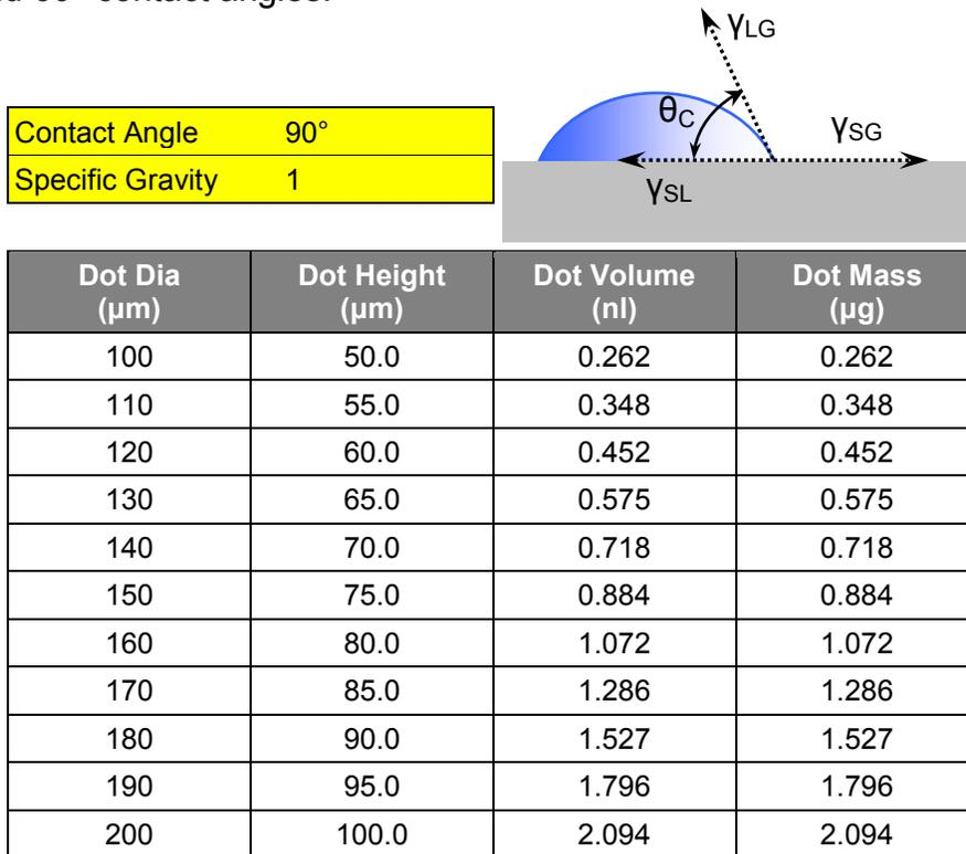
Figure A1 - 2: Guide to Selecting Nozzle Size
