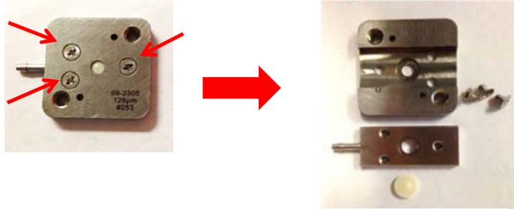
Figure 3-3: Disassemble the Nozzle Plate
