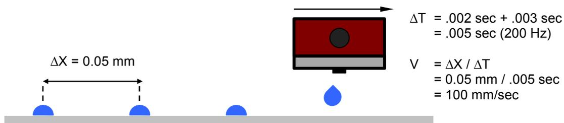
Figure A1 - 7: Calculating Robot Velocity for Drop Spacing = 0.05 mm, Refill Time = .002 Sec and Dwell Time = .003 sec
