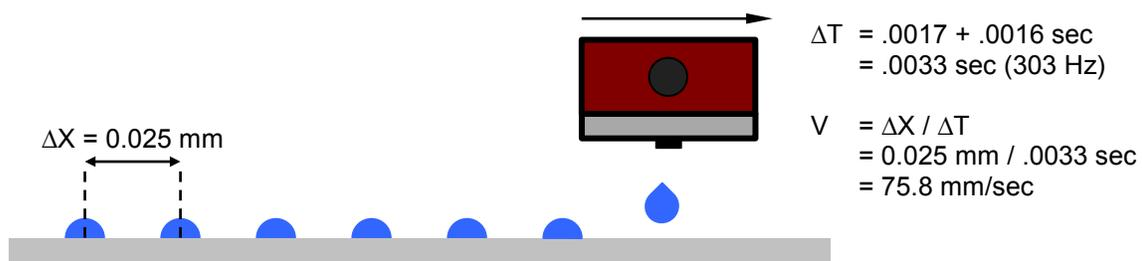
Figure A1 - 8: Calculating Robot Velocity for Drop Spacing = 0.025 mm, Refill Time = .0017 Sec and Dwell Time = .0016 sec
