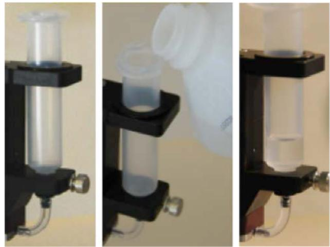
**Figure 4-2:** Install an Empty Syringe and Fill With Solvent
