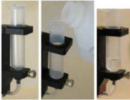
3. Fill the syringe with approximately 3 cc of mild solvent compatible with your fluid material. For example, use isopropyl alcohol to flush most underfill material, flushes, etc.
