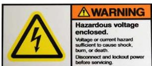
**WARNING: Live Voltages after Main Switch Off** - Any spare part replacement or maintenance work to be carried out on or near the components of the AC input line may only be started after the machine is disconnected from the AC supply (house line). These components carry dangerous electrical energy even when the main switch is turned off.
