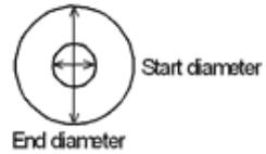
2. The head moves at Move Velocity to Settle Z and X, Y at the nearest point on the circle of diameter Start Diameter centered at X, Y.
