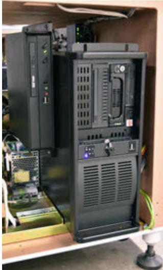
2. Secure the computer tower to the rack mount with four (4) screws.
