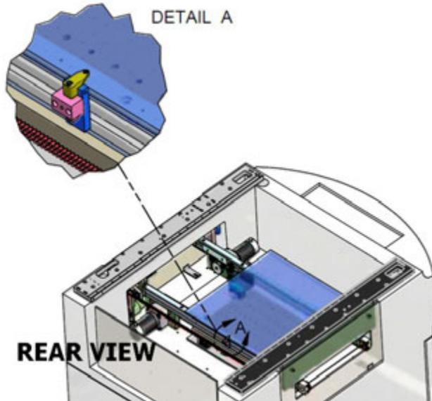
2. Secure the two, front, side clamps in the front slot of the front conveyor rail with the soft tips oriented toward each other at the designated distance (center-to-center) from each other:
