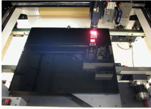
3. Adjust the position of the glass plate so its rows and columns of dots, not the plate edges, align with the work area. To fine tune glass position, refer to [Aligning Glass Plate to Gantry](#) (page 30).
