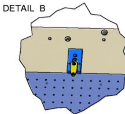
2. Similarly, secure the right-hand side clamp near the front right corner of the work area using the existing 6/32", tapped hole.
