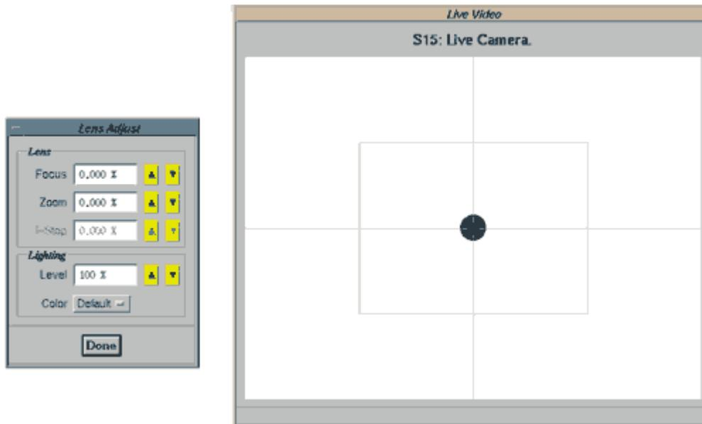
2. Adjust camera focus as needed using the arrows in Lens Adjust to obtain a clear picture in Live Video.
