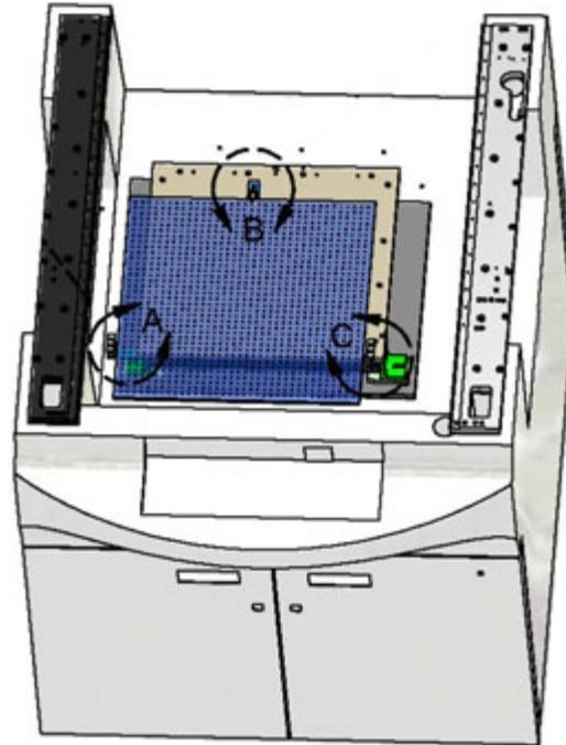
To install the three (3) glass plate clamps in a batch plate machine:
