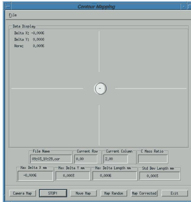
9. When the Delta X and Delta Y are as close to zero as possible (0.003 mm is acceptable), click DONE.
