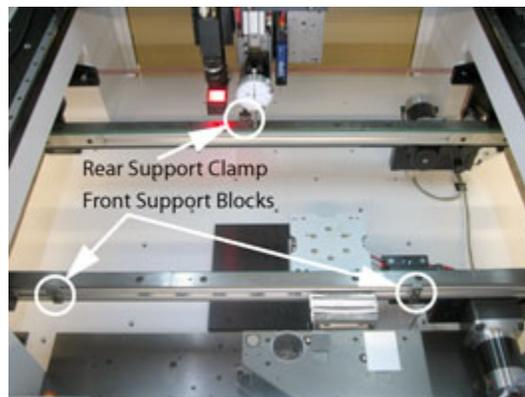
**NOTE:** The mapping kits are designed for use with *slotted* conveyor rails. In order for a mapping kit to be used with *solid* conveyor rails, a total of three tapped holes must be drilled in the rails.
