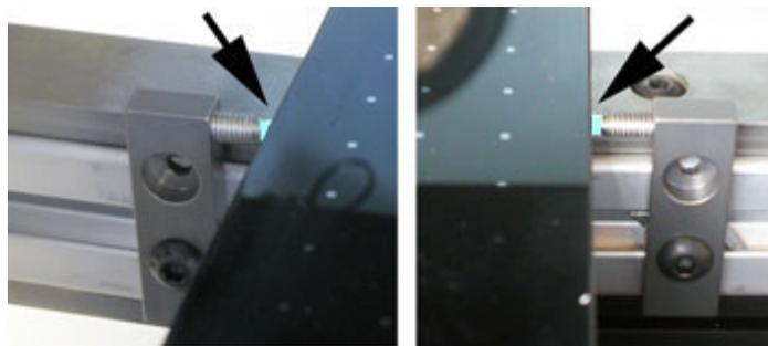
5. Carefully adjust the set screw (see below left) of the rear, top clamp so the plastic button (see below right) just contacts the glass plate.
