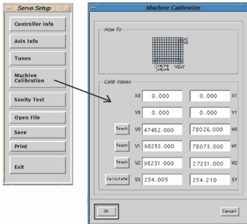
4. Teaching servo calibration requires the numbers of vertical and horizontal dots to be the same - a square pattern. The square (equal number of dots in X and Y directions) pattern should be as large as possible.
