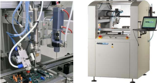
Both models are equipped with a robust 3-axis motion platform that, in the base configuration, includes a spray valve and a needle valve. An optional volumetric pump may be used in place of the needle valve.
