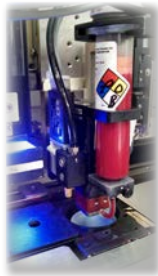
Direct Integration of NCM5000 Jetting Pump
