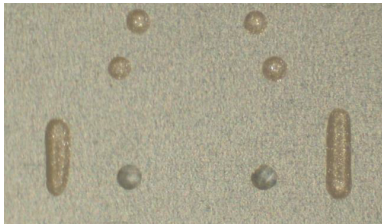
Structural and electrical conductive adhesives. Dots at 0.011" (0.27 mm).
