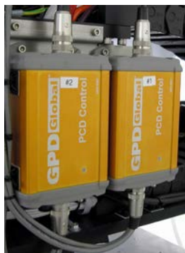
Figure 6: Two Control Interface units mounted on a machine
